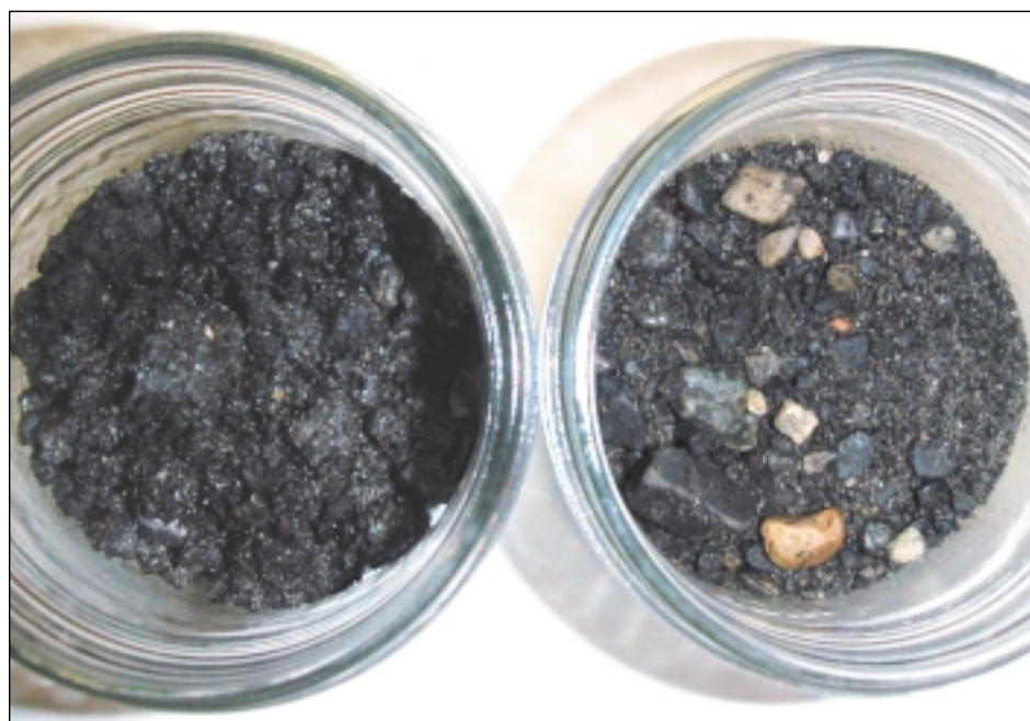
Pre and post treated oil-sands by-product wastes treated with Ivey-sol.
